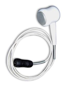
The ultra-sound wave is produced by a PIEZOELECTRIC TRANSDUCER: a special crystal that, when is subjected to an electric current, changes its form.
